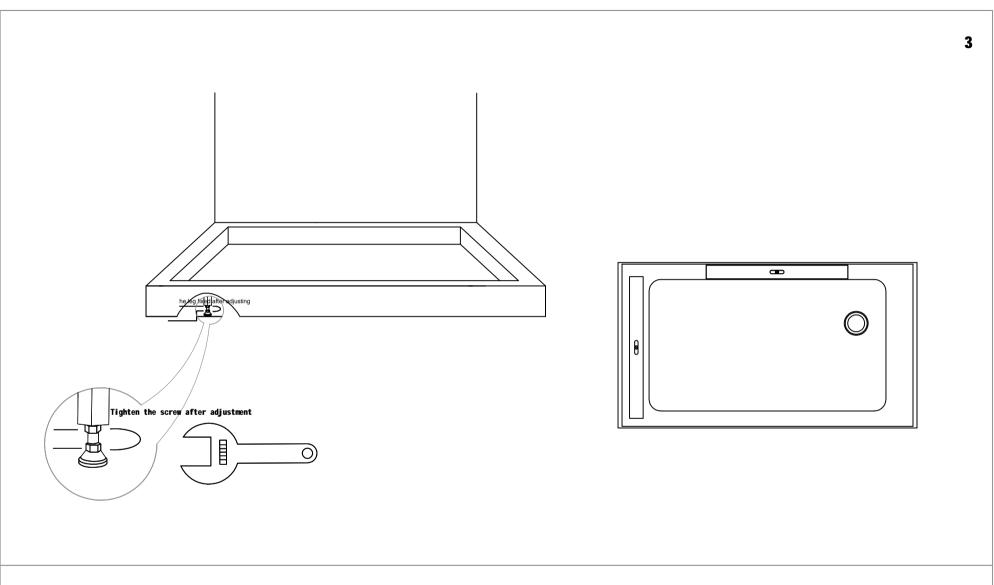
3.Adjust the shower tray: Insert the waster water pipe into the drain. Then adjust the foot of shower tray to keep the shower basin surface horizontal and perpendicular to the wall.
