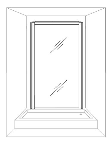
4.1 Put the shower tray to the installation place; 2 Put the glass of backboard against the wall.
