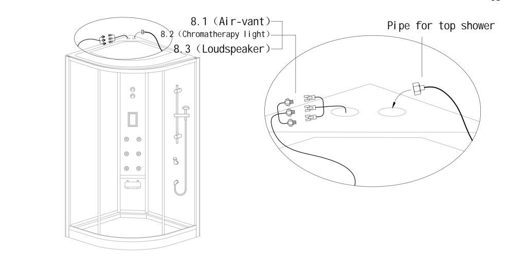
13. Connect the pipe for top shower and the pipes according to the number.
