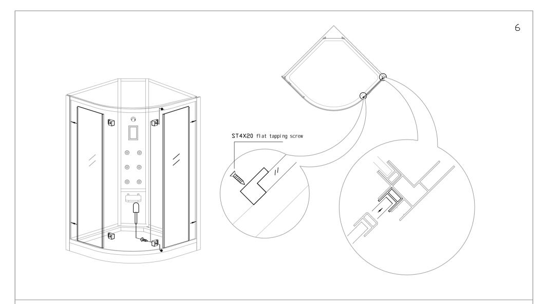
6. Install fixed glass door Get one side of the fixed door into door frame. Install the other side of the glass door onto the track with blocks on both ends through tapping screws.
