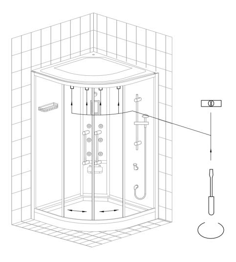
17. Adjust the gap between the cabin and wall:
