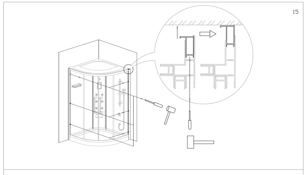
15. Push the cabin to the corner and adjust the profile as the drawing.
