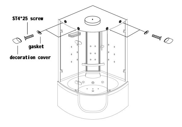
12. Fix the roof on the front glass with nut+ gasket M4\*25 screw.
