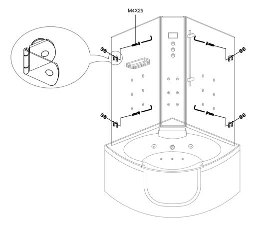
6.Install the connectors on the side backboards.
