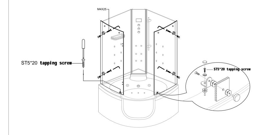
$7. \\lnstall$  the fixed glass: Connect the backboards and fixed glass with adjustable hinges. Then connect the fixed glasses with the cabin with bottom connector.
