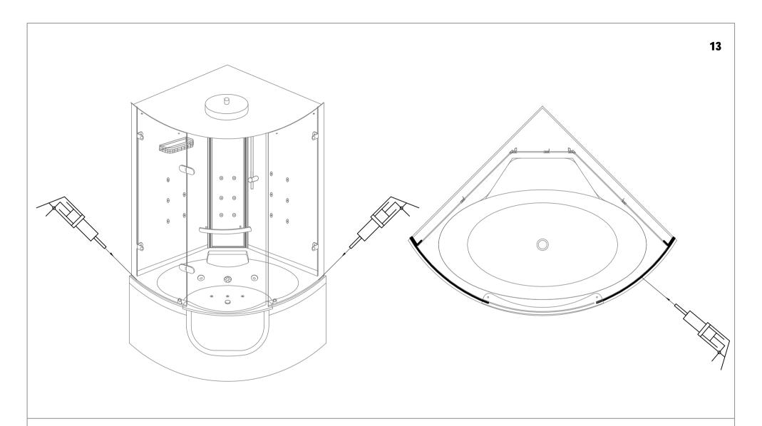
13.Installation finished. Apply silicone on the necessary position. Connect the power supply, water supply, floor drain, ground wire and then push the cabin to the corner. Don't use the cabin until the silicone is dry.
