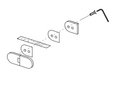
$8. \, \text{Install} \,$  the hinge on the left side fixed door.
